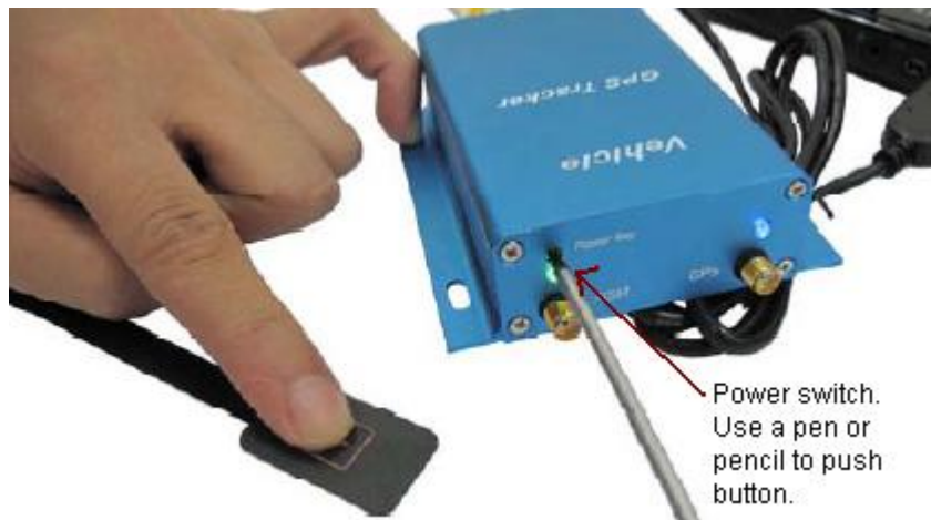
Figure 8: Power On Modem for Configuration
